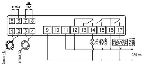
The sensor S1 (black) must be in the ambient. The sensor S2 (gray) must be placed in the evaporator through metallic clamp.
