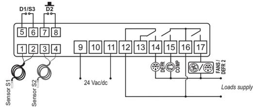
The sensor S1 (black) must be in the ambient. The sensor S2 (gray) must be placed in the evaporator through metallic clamp.
